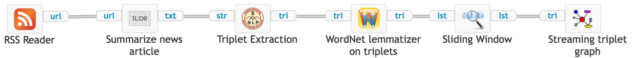
Figure 5: The semantic triplet graph from an RSS feed workflow constructed in the CloudFlows platform. The workflow is publicly available at http://cloudflows.org/workflow/1729/ .
